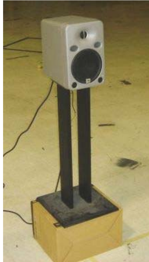
Fig. 92a. A JBL model LSR 25P powered mini monitor mounted on a stand. The height of the monitor was raised so that its axis was 1 m high (a point midway between the tweeter and woofer). This system was measured to illustrate the frequency response effects of operating a conventional speaker system over a reflective ground plane.
